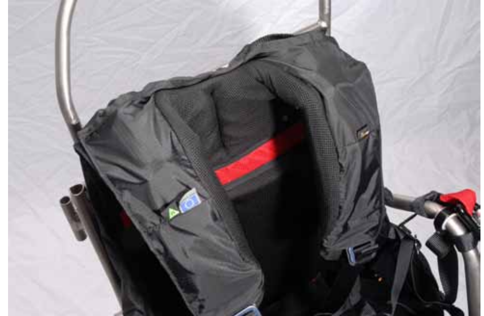
When the installation is completed : close the risers flap covers to tidy up the harness.
